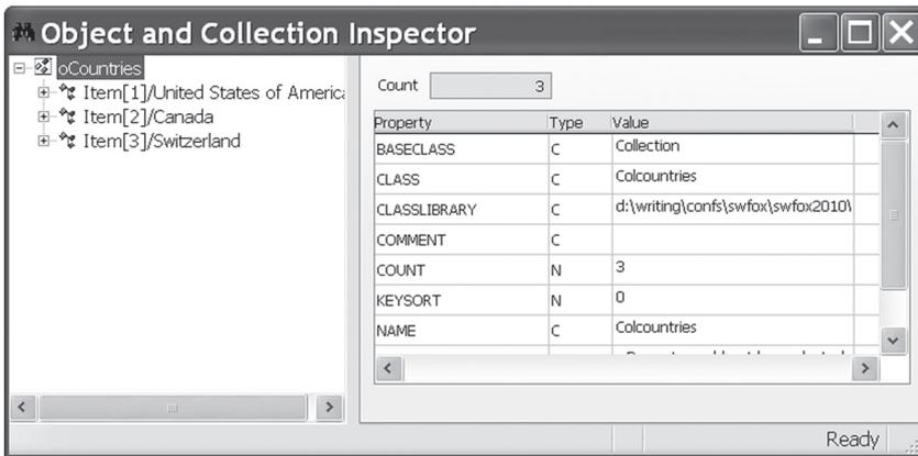
**Figure 2.** When you drill into a collection, each item is shown with its index number and, if it has one, its key.
