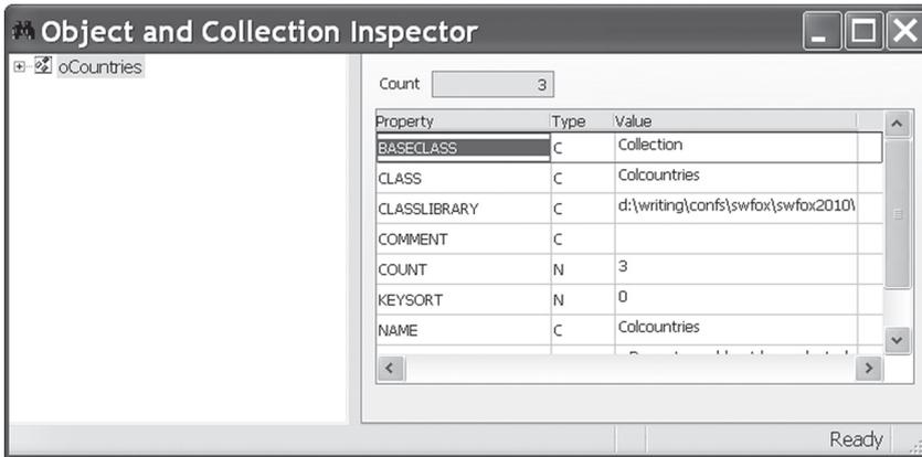
**Figure 1.** For a collection, the Object Inspector shows the count and then all the properties of the collection.
