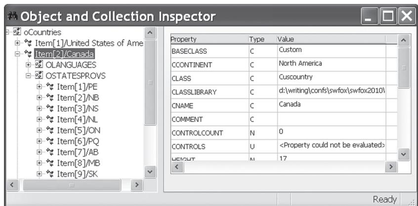
**Figure 3.** Click on a member of a collection to learn more about it. For objects, the right panel shows the object's properties and their current values. In this figure, the oStatesProvs collection inside the object has also been expanded.
