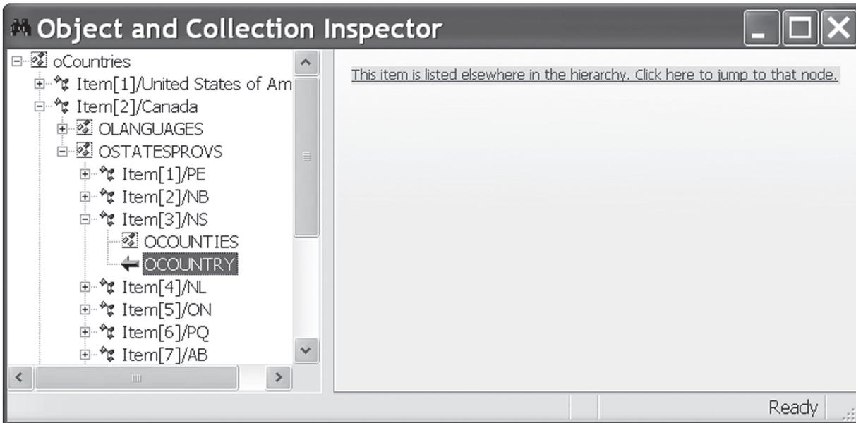
**Figure 5.** When a hierarchy contains cycles, only the first occurrence of an object appears in the right panel. Subsequent occurrences give you a link back to the first instance.
